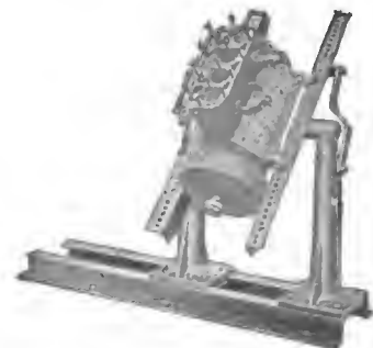
Every-Way engine stand, showing mounting of engine
